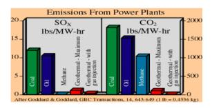
Fig. 1: A comparison of Greenhouse emission from power plants
