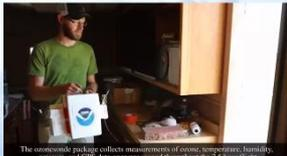
The radiosonde package collects measurements of ozone, temperature, humidity, pressure, and GPS data once per second throughout the 2.5 hour flight.
