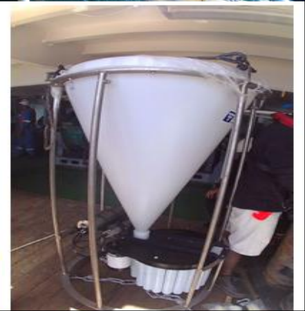
Sediment traps – measuring what falls down to the ocean bed over one year
