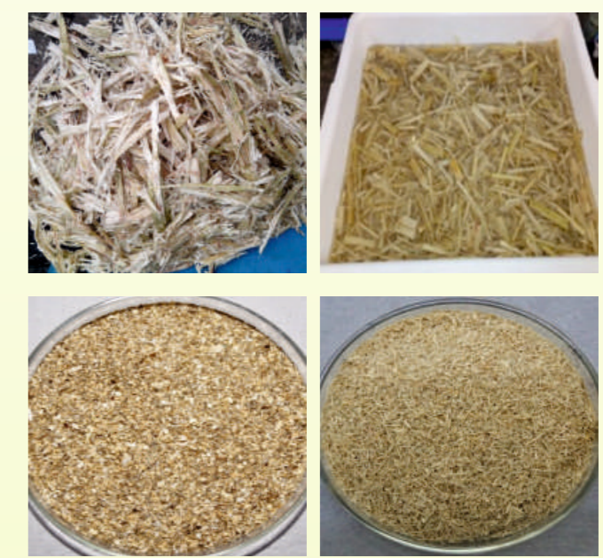
Biosorbent (Sugarcane Bagasse (A) and washed (B) & Peanut hull (A) and Sugarcane Bagasse (B) after grinding and sieving
