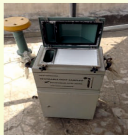
RESPIRABLE DUST SAMPLER (PM 10 )
