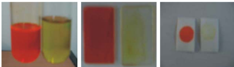
Fig. 1: Photographs of the polymer solution (a), polymer film on glass substrate (b) and polymer film on filter paper (c) before and after exposure to \text{NO}_2 gas. In all the cases the original orange color is bleached to pale yellow on exposure to \text{NO}_2 gas.
