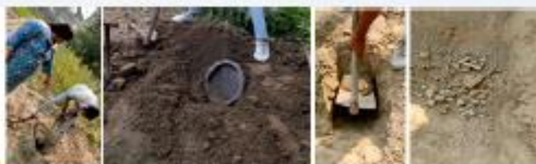
Biodegradable Plastic Products 100 % degraded within 60 days under Soil conditions
