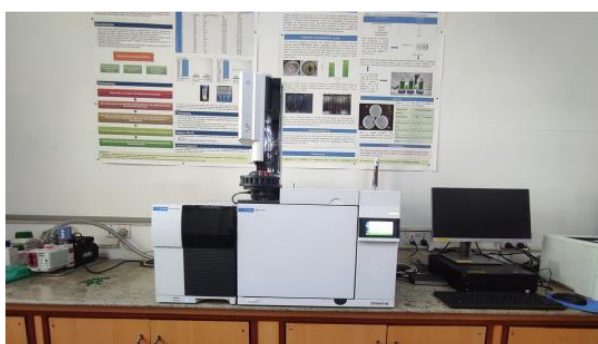
GC and GC/MS Facility
