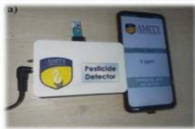
OP detection Hand-held sensor with plugged in OP probe and connected to mobile phone by BLE
