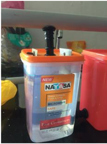
Fig. 6. Cell containing copper and zinc electrodes
