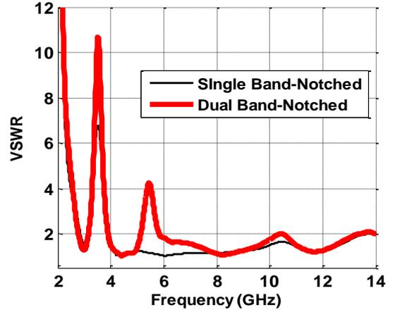
Fig. 4 Simulated VSWR of DBN-UWB Antenna.
