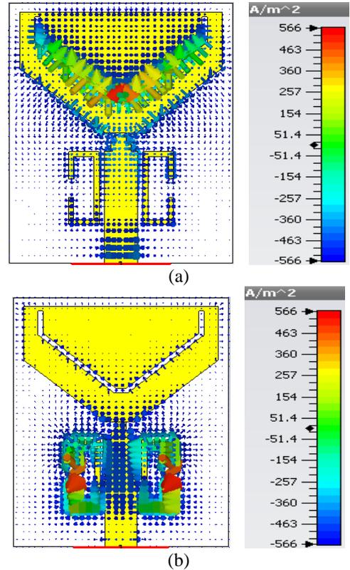
Fig. 5 Surface current distribution at (a) 3.5GHz and (b) 5.5 GHz.
