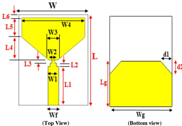
Fig. 1 Proposed Basic Trapezoidal UWB antenna structure design.
