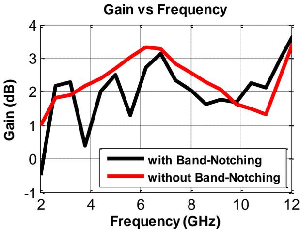
Fig. 7 Gain comparison of proposed basic UWB & DBN-UWB antennas.
