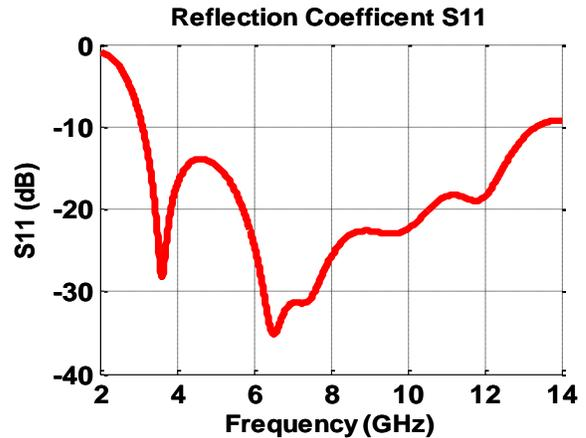
Fig. 2 Simulated Reflection Coefficient of Basic UWB.
