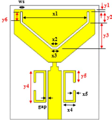
Fig. 3 Proposed DBN-UWB antenna structure top view.
