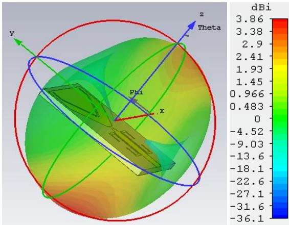
Fig. 6 3D view of Directivity at 6.5GHz.
