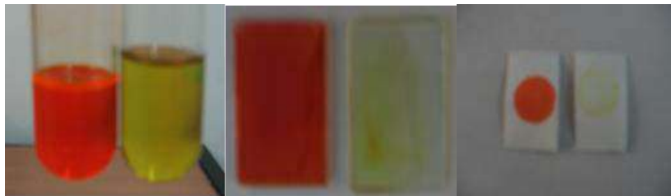
Fig. 1 Photographs of the polymer solution (a), polymer film on glass substrate (b) and polymer film on filter paper (c) before and after exposure to NO 2 gas. In all the cases the original orange color is bleached to pale yellow on exposure to NO 2 gas.
