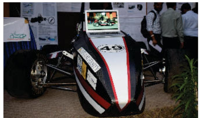
An innovative device **"Design and Fabrication of Bodyworks of Formula Car by Carbon Fibre Resin"** by Mr. Abhishek Mehta, Mr. Kush Prakash Srivastava, Mr. Srinivasana and Mr. Bellam Jayanth of B.Tech Mechanical Engineering. The design of the bodywork is made using the Autodesk software named FUSION to produce the detail 3D design.
