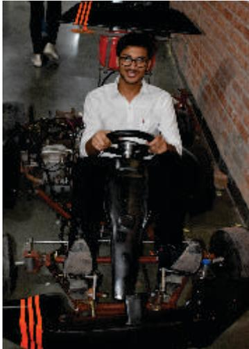
An innovative device **“Design and fabrication of drive train and transmission system of Go-Kart”** by Mr. Faisal Khan Afridi, Mr. Lokesh Pal, Mr. Bilal Khan and Mr Zubair Ahmad Shalla of B.Tech Mechanical Engineering. The device is designed and fabricated, which is characterized by the absence of differential and suspensions systems.
