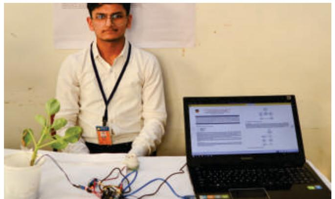
An innovative device **"Automatic Plant Watering System using IoT"** by Mr. Eish Mital and Ms. Shikha Guleria of B.Tech - Information Technology. This system has a soil moisture sensor and relay connected to the Arduino board.
