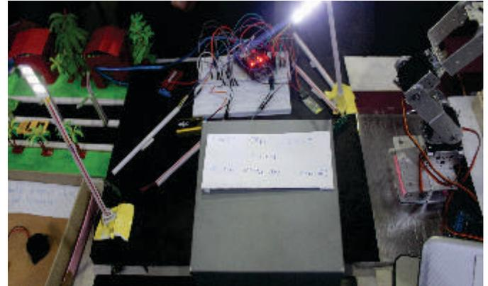
An innovative device **"Smart Street Lighting"** by Mr. Aditya and Mr. Anish of B.Tech Electronics and Communication Engineering. The smart lighting system is based on the movement recognition of traffic and the ambient light intensity on road in order to control the LED street lighting using the dimmer circuits and sensors.
