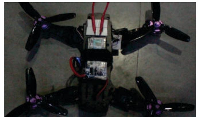
A project **"Remote controlled Courier Drone with load pickup and drop mechanism"** by Mr. Pushkar Singh of B.Tech Electronics and Communication Engineering. It is a remote control quadcopter consisting of F3 flight controller known as the mind of the drone.
