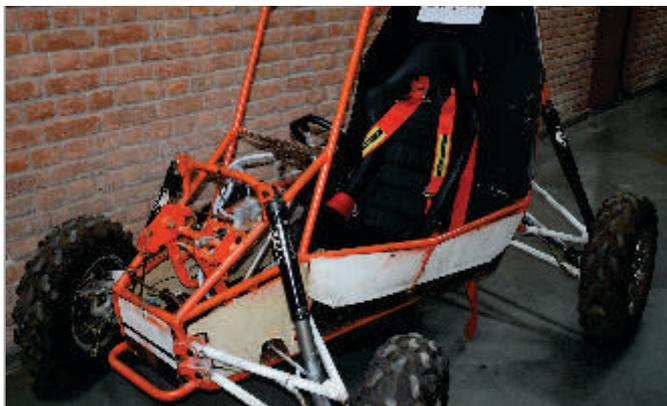
A project **"Suspension Brakes & Steering Hub Assembly for ATV"** by Mr. Sumit Kapri, Mr. Sheesh Gupta and Mr. Saurav Kumar, B.Tech Mechanical Engineering. Single passenger, off-road vehicle powered by a 10 HP Briggs & Stratton of 305cc engine.
