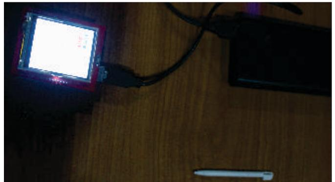
11. A device **"Digital Notebook for Academic Purposes"** by Mr. Venu Acchaand, Mr. Raj Tirtha of B.Tech Electronics and Communication Engineering. The device consists of a touch screen interface on which a user can write using a stylus.
