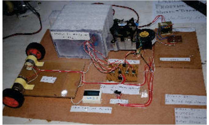
A project on **"Thermal Management of Li-Ion Battery Array Arrangement in Electric and Hybrid Vehicle Application"** by Mr. R Umesh, Mr. Hemant Tanwar, Mr. Aman Singh Purbiya and Mr. Ranjan Prabhu of B.Tech Mechanical Engineering. The device controls nano surface heat transfer rate between the lithium-ion batteries.
