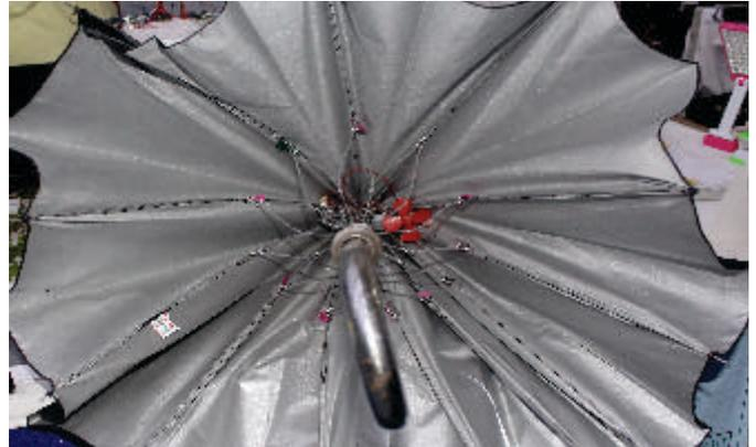
A project **"Solar Umbrella with Attached fan, Charging Point and Torch"** by Ms. Sonal Gupta and Mr. Mayank Agarwal of B.Tech Electronics and Communication Engineering. A solar umbrella is made with attached solar panels on the top and battery connected to it as a solution of this problem. The umbrella is even connected with a fan, a charging point and also a torch.
