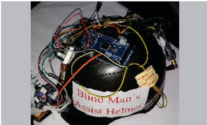
An innovative device "Blind man Assisting Helmet" by Mr. Vanacharla Bala Sai Mohan, Mr. Yadla Rishi Kiran and Mr. Kshitij Gupta of B.Tech Electrical and Electronics Engineering. The device is designed for the purpose of navigation using the ultrasonic sensor and a servo motor.
