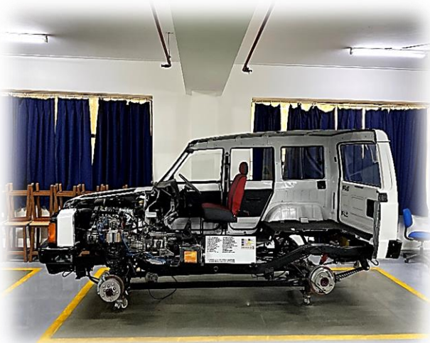
Cut Section of Diesel Engine of Tata Sumo in Automobile Engineering Lab
