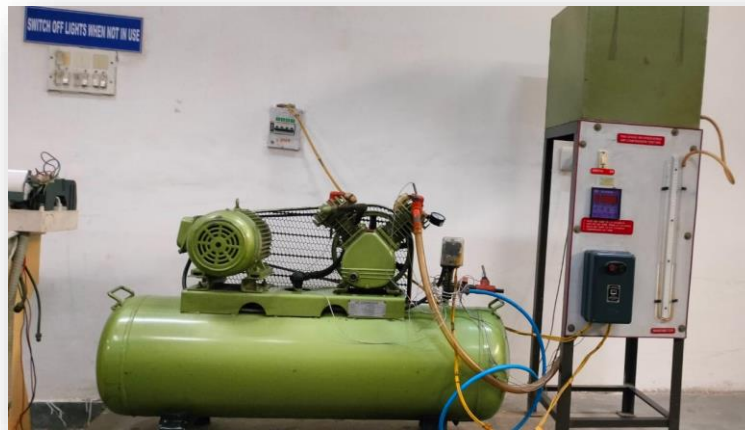
Reciprocating type multi cylinder air compressor facility
