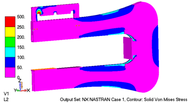
Fig. 12. Maximum Stress are coming < 150Mpa
