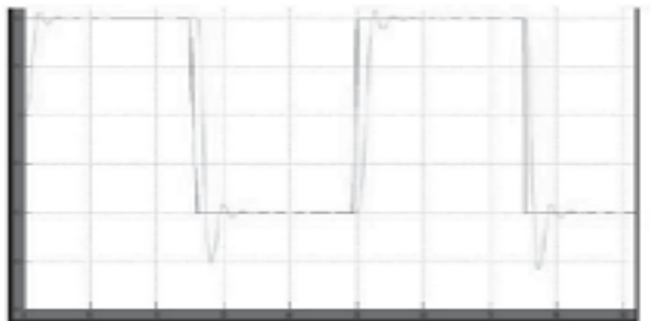
Fig. 14. TRMS Control system response for square input
