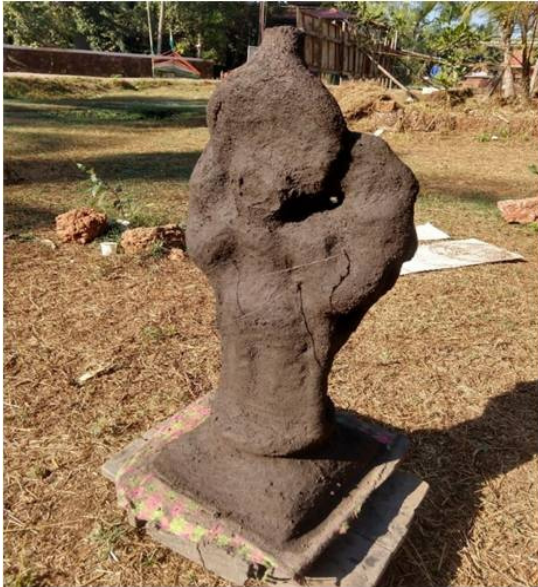
Fig. 9. Moulds is place under the sun for initial dry process.
