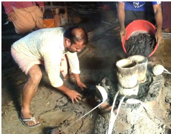
Fig. 13. Traditional furnace with coal firing for melting the metal.
