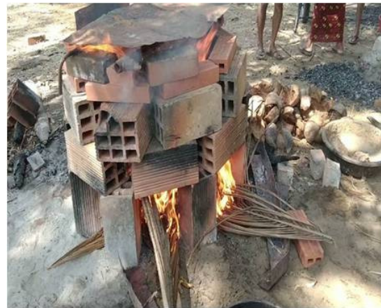
Fig. 12. Final firing of moulds for the complete De-waxing.
