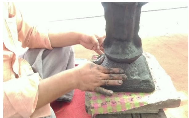
Fig. 6. First layer of mould making process with fine clay.
