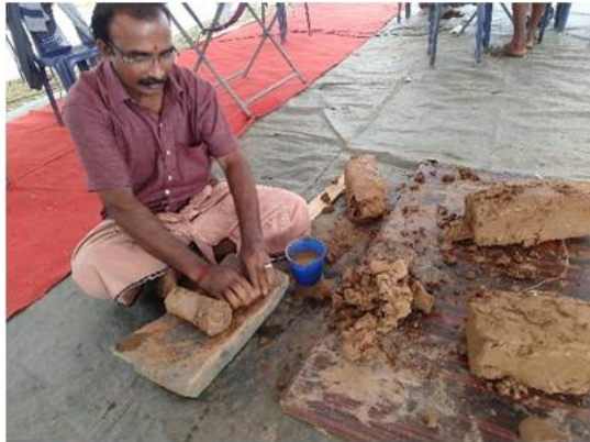
Fig. 5. Preparation of clay for mould making process.
