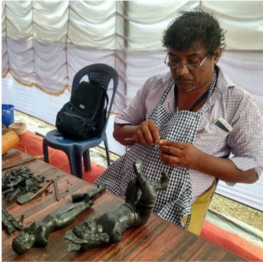
Fig. 3. Wax modelling using a knife and scraper.
