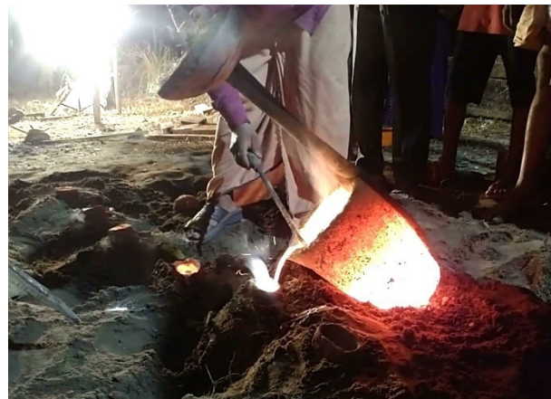
Fig. 14. Pouring of molten metal into the moulds, buried in the ground pit with mould pouting mouth facing out upwards.
