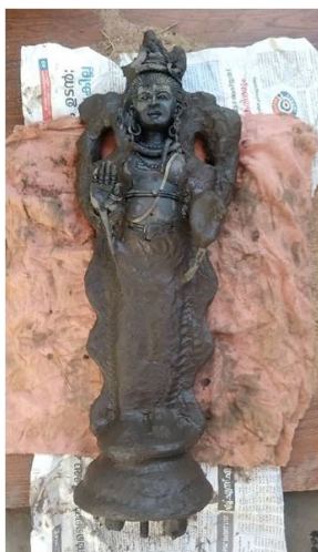
Fig. 7. While mould making process, Wax model is kept on piece of cloth.
