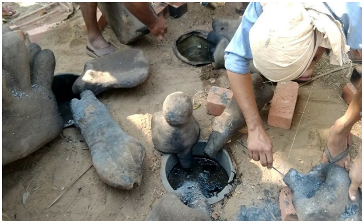
Fig. 11. Mould are place on a vessel to collect the wax.
