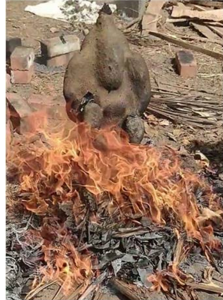
Fig. 10. Initial de-waxing process by open firing.
