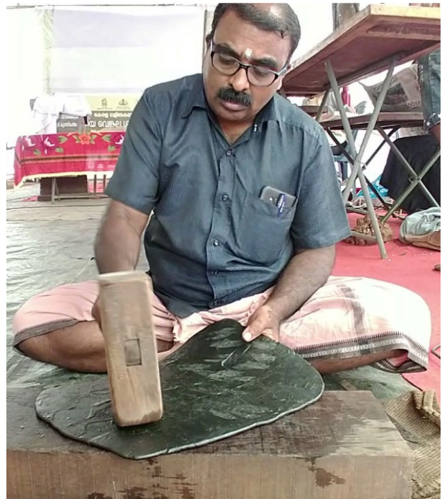
Fig. 2. Creating Wax sheet by beating it with wooden mallet.
