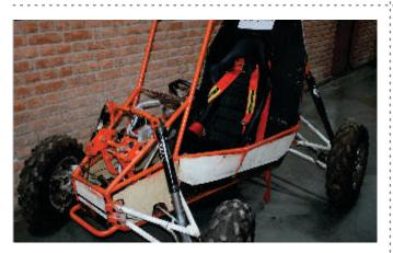
A project **"Suspension Brakes & Steering Hub Assembly for ATV"** by Mr. Sumit Kapri, Mr. Sheesh Gupta and Mr. Saurav Kumar, B.Tech Mechanical Engineering. Single passenger, off-road vehicle powered by a 10 HP Briggs & Stratton of 305cc engine.
