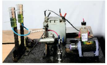
A novel project **"Effect of ambient parameters on exhaust of 2 stroke engine"** by Mr. Tushar Gupta, Mr. Vipul Tyagi and Mr. Nitin Kaushal of B.Tech Mechanical Engineering. This project work aims at studying the exhaust of 2 stroke engines and reducing their harmful residual gases and improves its performance for better outputs.
