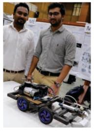
Design and fabrication of pneumatic car bumper A state-of-the-art project by Fazil Hafeez, Jomin Johnson, Anant Chaturvedi and Gokul Mohan of B.Tech Mechanical Engineering. A design of pneumatic piston car bumper based on the pneumatic control of the movable bumper. The bumper attenuates collision energy thereby decreasing the collision damage to the car and passengers.
