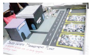
Segregation of Organic and Inorganic Matter in MSW with Air Density Separator Umanath P Shenoy and Amanuddin Hamidi of B.Tech – Civil Engineering designed an Air Density separator that uses an air current to separate a material from another of greater density or particles from other greater size or shape
