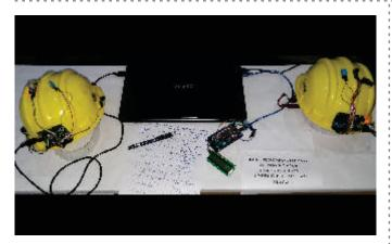
A project on **"Real time Monitoring of hazardous parameters in underground coal mines"** by Mr. Akshunya Mishra, Mr. Saksham Malhotra, Mr. Nishant Kumar Sinha and Mr. Harsh Bardhan of B. Tech Electrical and Electronics Engineering. This system is designed for the safety measures in an underground coal mines.
