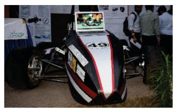
An innovative device "**Design and Fabrication of Bodyworks of Formula Car by Carbon Fibre Resin**" by Mr. Abhishek Mehta, Mr. Kush Prakash Srivastava, Mr. Srinivasana and Mr. Bellam Jayanth of B.Tech Mechanical Engineering. The design of the bodywork is made using the Autodesk software named FUSION to produce the detail 3D design.
