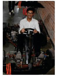
An innovative device "Design and fabrication of drive train and transmission system of Go-Kart" by Mr. Faisal Khan Afridi, Mr. Lokesh Pal, Mr. Bilal Khan and Mr Zubair Ahmad Shalla of B.Tech Mechanical Engineering. The device is designed and fabricated, which is characterized by the absence of differential and suspensions systems.
