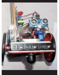
An innovative project **"An EMP Jamming Robotic System using Arduino Programming"** by Mr. Karush Suri and Mr. Mohit Mehta of B.Tech Electronics and Communication Engineering.
