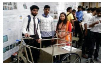
**To Design and Fabricate E-Tricycle for Physically Handicapped** Work for a cause - A project by Aklavya, Shanky, Ishaan and Gaurav Singh of B.Tech Mechanical Engineering. A transportation vehicle designed for physically disabled persons especially with crippled legs for easy mobility.
