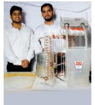
A project **"Multi-evaporator** system for cleaning of water using wastage heat of the plant" by Mr. Pushkar Singh of B.Tech Mechanical Engineering. The purpose of this project is to treat rejected RO water through multi evaporation and make use of this rejected
