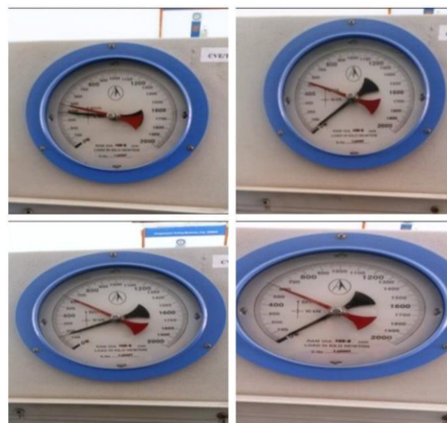
Figure 6: Compressive Readings of Cubes
