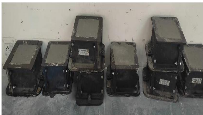
Figure 5: Cubes Casting of M20 Grade of Concrete
