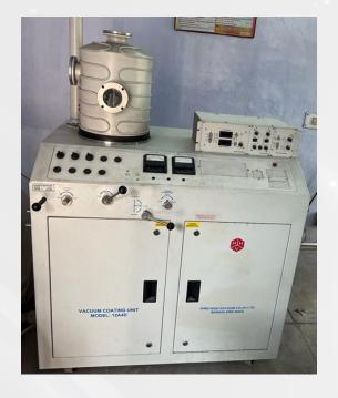
Equipment 12: Electron Beam Physical Vapour Deposition (EBPVD)
